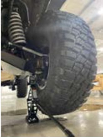
Example of jack placement on the outboard end of the Lower Control Arm.
