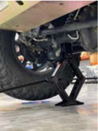
Example of jack placement on the OEM Rear Axle Housing Tube.
